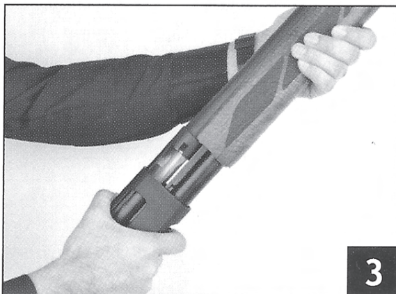
3 - Remove forend & barrel assembly together by pulling forward.
